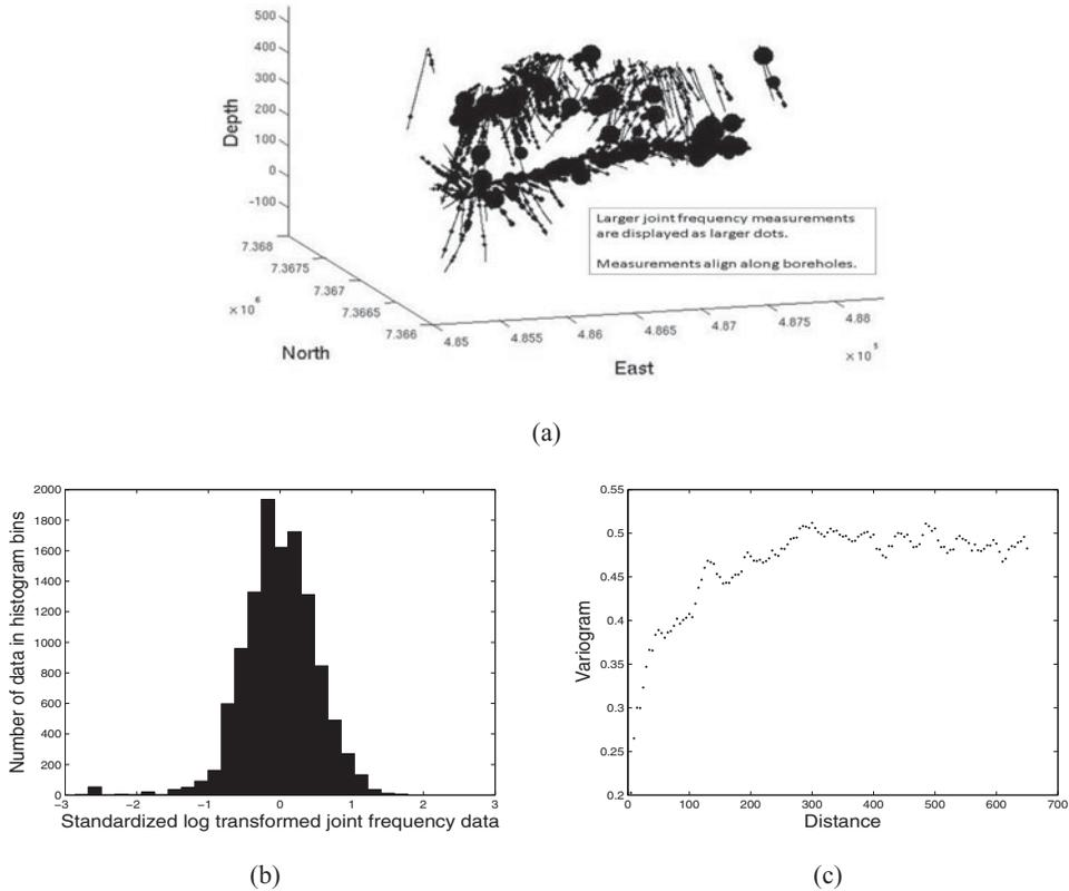
Figure 4. Mining data: (a) Data sites in a Norwegian iron mine. The data size is  $n = 11,107$ , collected in about 200 boreholes. (b) Histogram of shifted log-transformed data of joint frequencies. (c) Empirical variogram.
